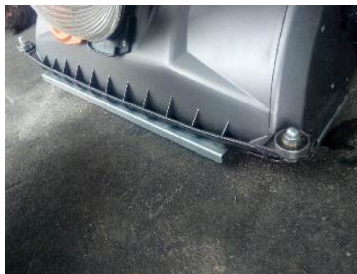
Fig.30-2 The baffle is inserted into place
