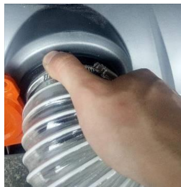
Rotate the hose connector clockwise to secure
