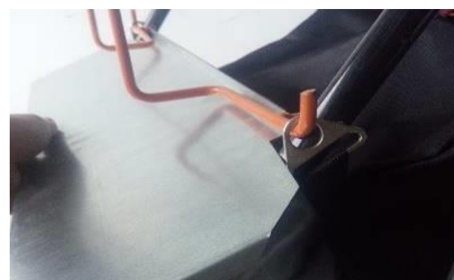
Fitting the baffle plate to divert the suction through the hose
